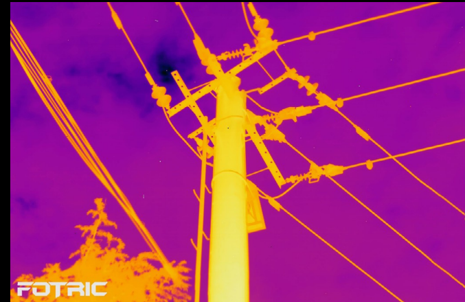
1280*1024 IR resolution (25° lens at 30m distance)
